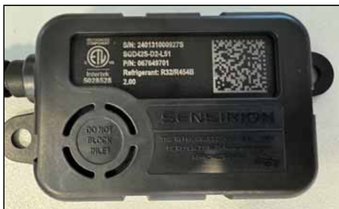
FIGURE 22. Example of Clear, Unobstructed Sensor Inlet
