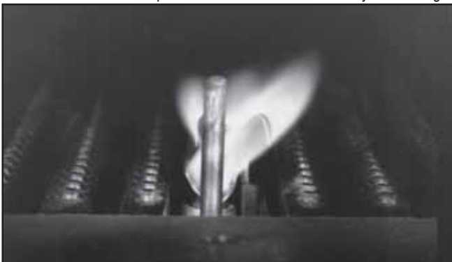
Figure 7. — Pilot Flame Pattern (Standard Burner)
