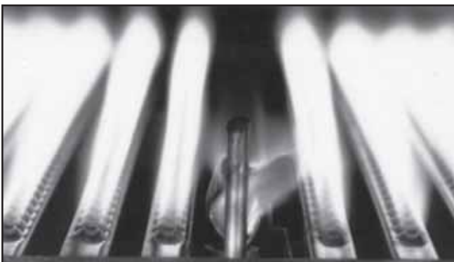
Figure 8. — Pilot & Main Burner Flame Pattern (Standard Burner)
